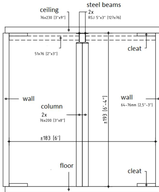
Figure 6: Structure of the central tunnel of the Zonnebeke Dugout (Ingenieursbureau Norbert Provoost bvba)
